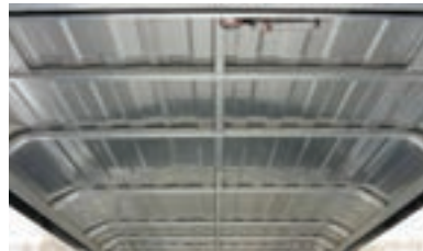
TIG Welded Super Cage Roof Integrated Construction
