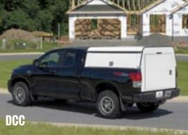
• 23" Height Cap • Full Length Side Door • Single Full Rear Door • Stainless Steel T-Handle Bolt Locks
